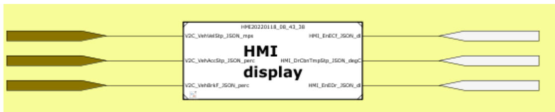
Figure 32: HMI Display interfacing
